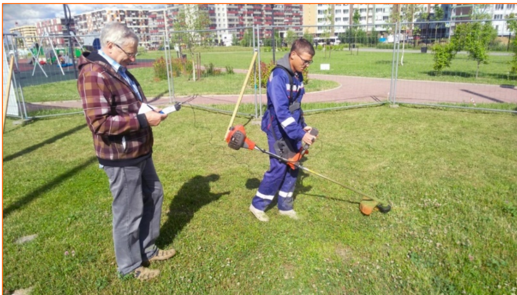
Figure 2. Process of Husqvarna 525RX octave spectrum vibration speed measuring.
